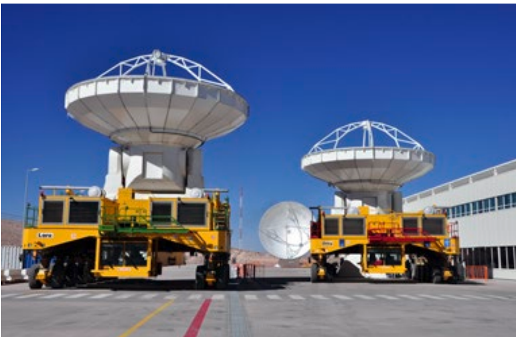
Image 9. Otto and Lore, the ALMA antenna transporters, in action. Credit: ALMA (ESO/NAOJ/NRAO).
